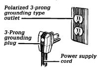
The compactor is for use on a single phase, 115-volt, 60 Hz, AC only 15 or 20 ampere fused and properly grounded circuit and is equipped with a grounding plug as shown above. Time delay fuse or
